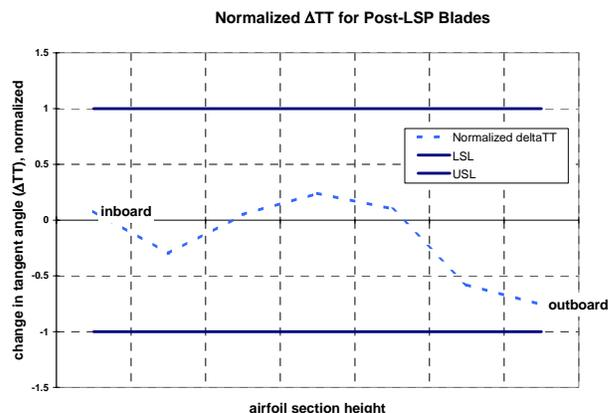
**Fig. 14 Normalized change in airfoil tangent angle post-LSP for treated fan blades**
