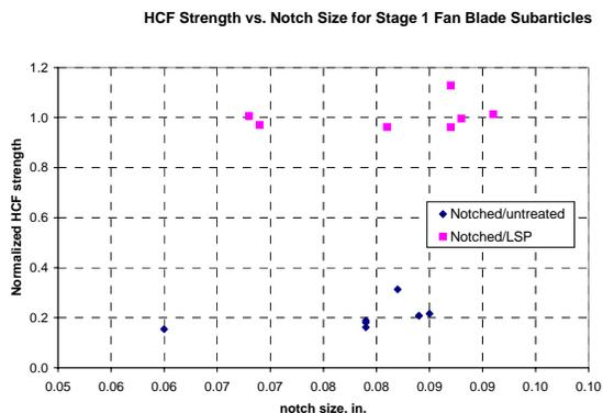
**Fig. 12 Relationship of HCF strength versus imposed FOD notch size**
