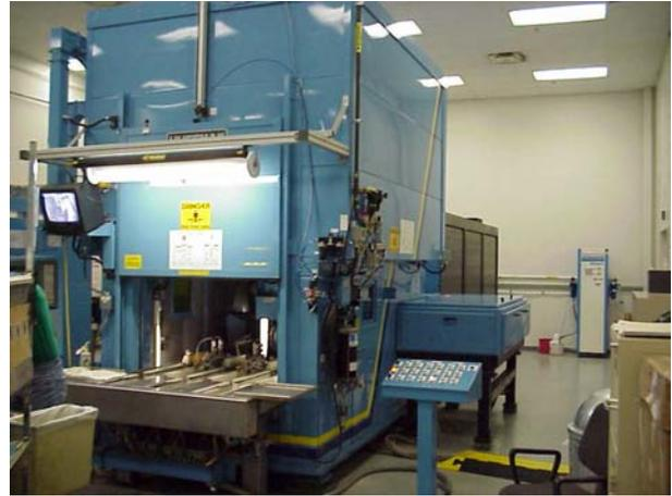
**Fig.4 Gen II laser shock peen apparatus**
