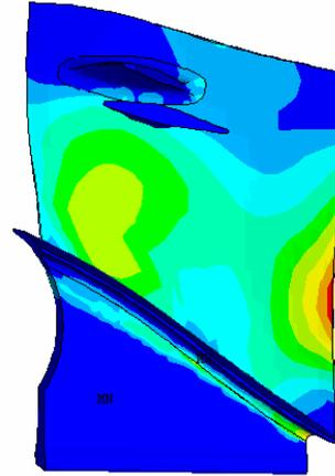
**Fig. 7 Normalized effective stress contours for first flexural (1F) mode of fan blade subarticle**
