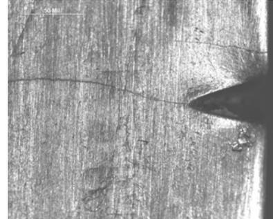
**Fig. 17 Crack propagated from notch during siren testing of LSP sample**
