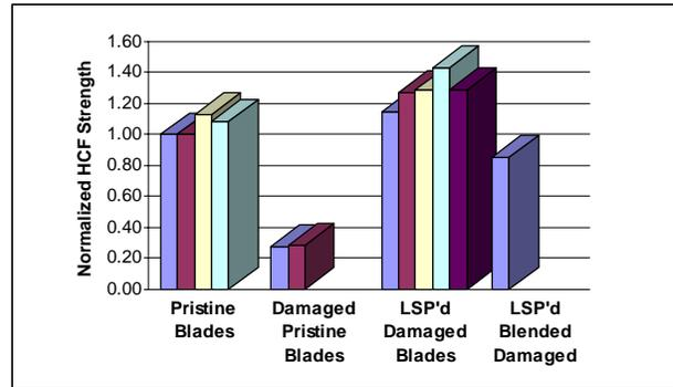
**Fig. 2 Typical fatigue capability comparison for Ti 6Al-4V fan blades using GEAE's Gen II technology**
