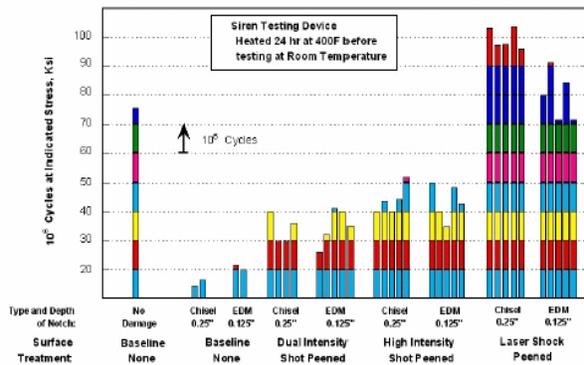
**Fig. 1 Comparison of HCF capability for various conditions for a Ti 6Al-4V fan blade<sup>3</sup>**
