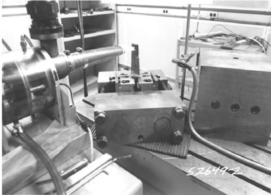
**Fig. 9 Typical setup for strain distribution/siren testing**
