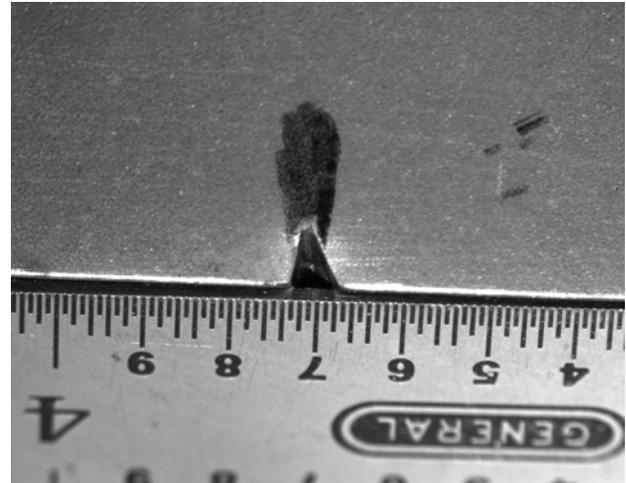
**Fig. 10 Stage 1 fan blade subarticle sample notch used to simulate LE FOD**
