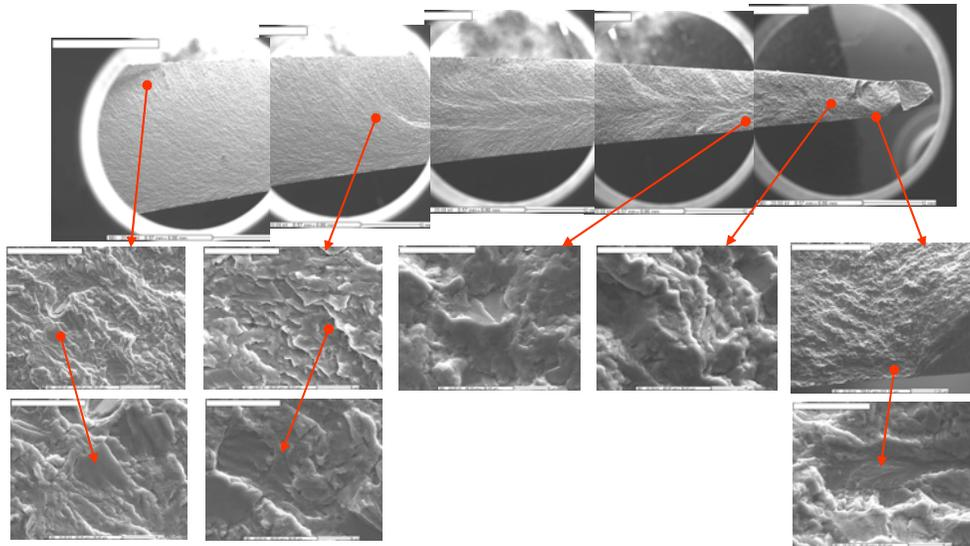
**Fig. 18 Fractography of sample after HCF testing**
