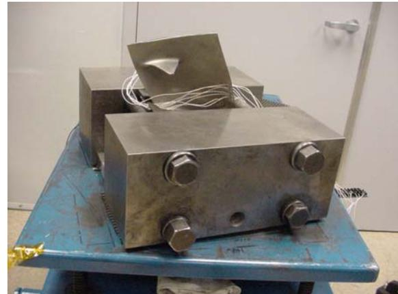
**Fig. 8 Blade subarticle setup for strain distribution/siren testing**
