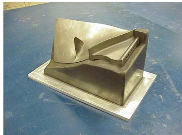
**Fig. 11 Fixture to secure fan blade for LE notching operation**
